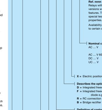
Basic identification principle (type designation code electromechanical relays)
