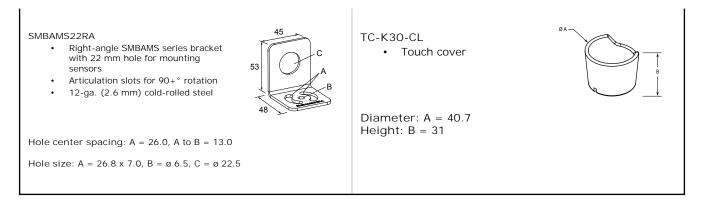
All measurements are listed in millimeters, unless noted otherwise.
