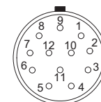
Counting direction cw (e.g. female connector)
