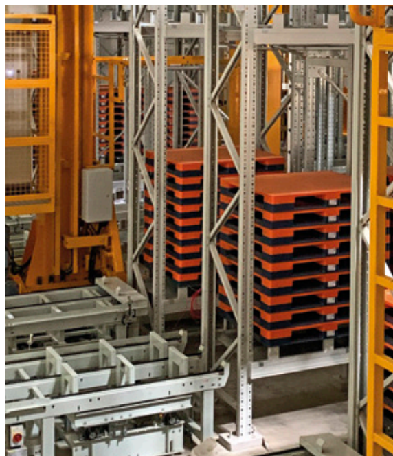
The TN-Q175 RFID reader is used where up to nine stacked empty pallets are read simultaneously
