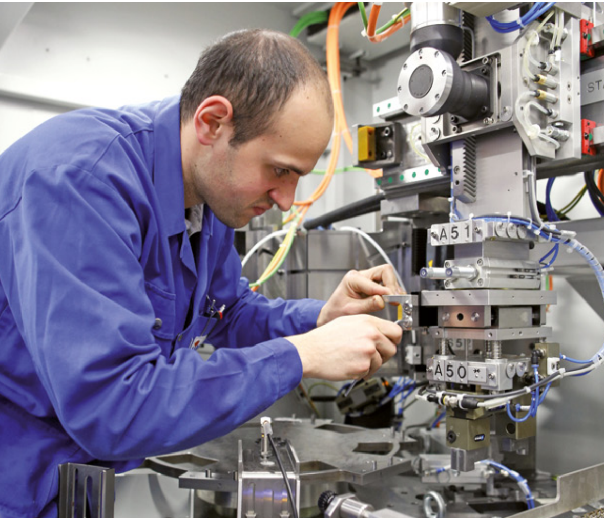
For a customer from the automotive industry, Linear Abrasive built the machine for grinding connecting rods with continuous parts machining on both sides
