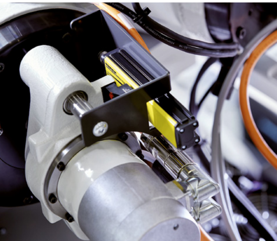
Turck's Li-Q25 sensor meets Arburg's demanding requirements in terms of positioning accuracy and reproducibility
