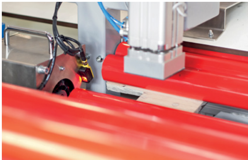
The Q20EQ7 infra-red sensor detects the joint between two pipes
