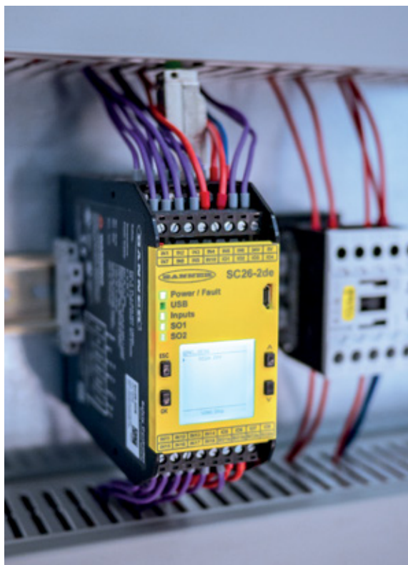
Banner's SC26-2 safety controller controls the safety functions of the machine
