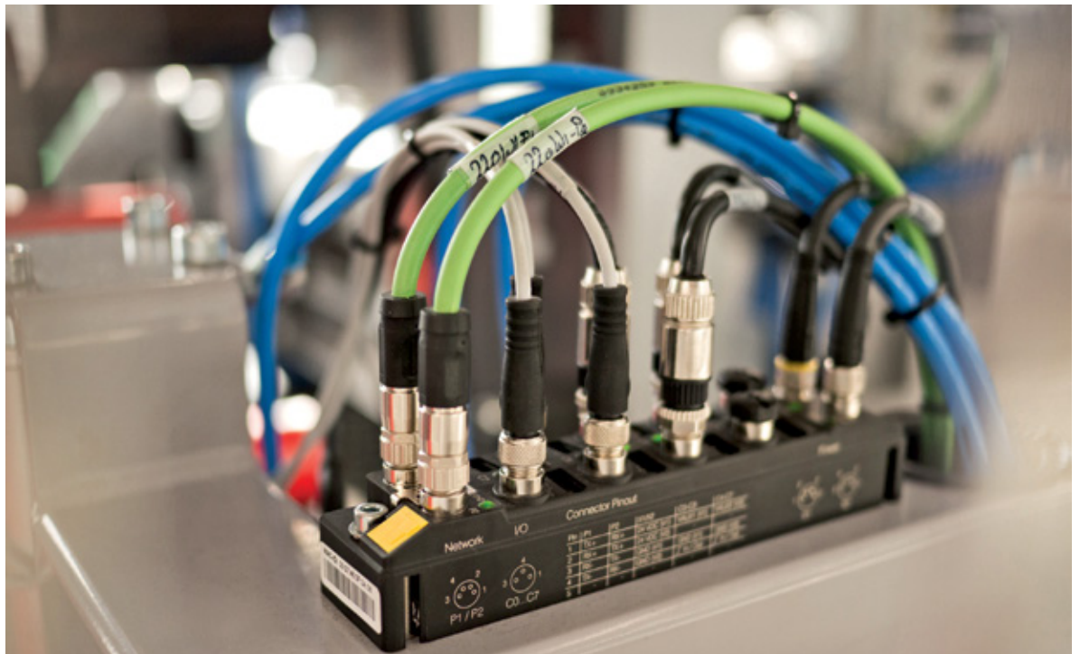
The TBEN-S I/O modules route all the signals to the controller via Profinet
