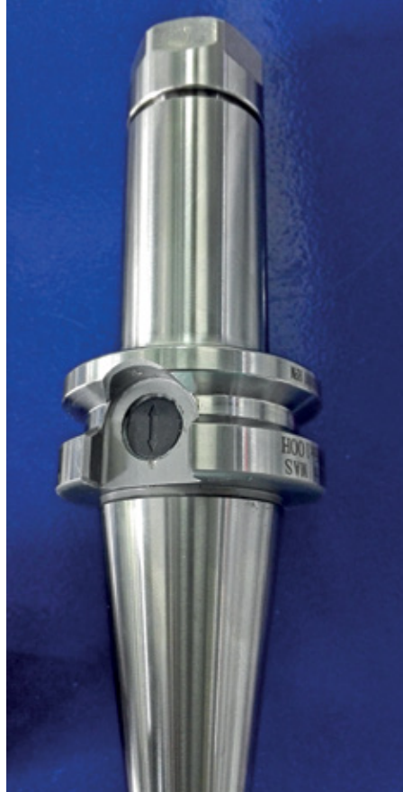
Cutting tool holder with embedded RFID tag
