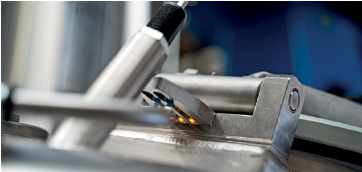
Compact BIM-UNT magnetic field sensors are concealed in the fill openings
