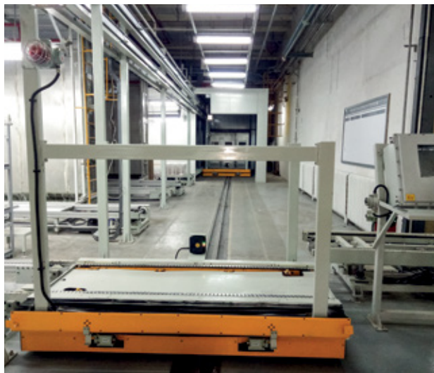
The moving rail transporter uses the Q175 reader to find out the section in which the individual workpieces are to be assembled
