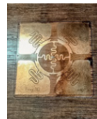
RFID inlays are inexpensive data carriers for complex process chains
