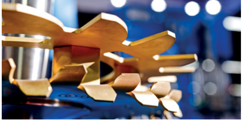
During the production process a double suction disc in the container rotates at the set height
