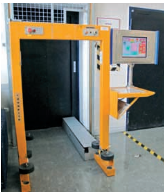
While the destination is keyed into the control pad, the RFID reader (bottom right) identifies the container
