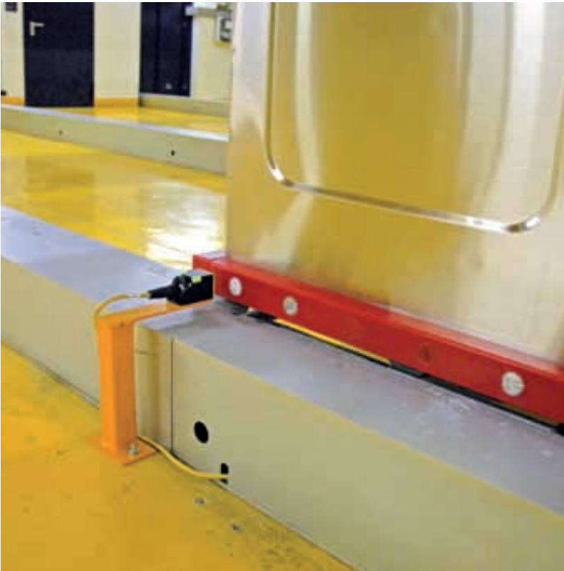
The reader reads the RFID tag that is screwed into the protection strip
