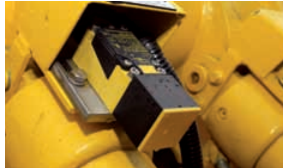
To measure position in their offshore drilling rig, Streicher uses inductive Namur-sensors with a high operating distance from Turck. Page 26
