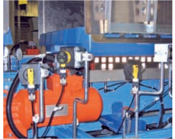
Smart: The ball-and-socket joint rack allows an alignment in X and Y direction
