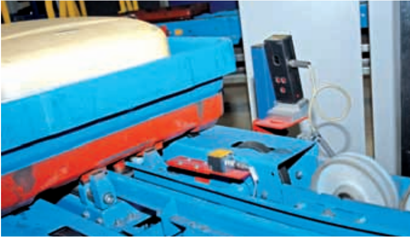
The reading station that Turck built for SEAP Automation contains a light sensor and three light barriers
