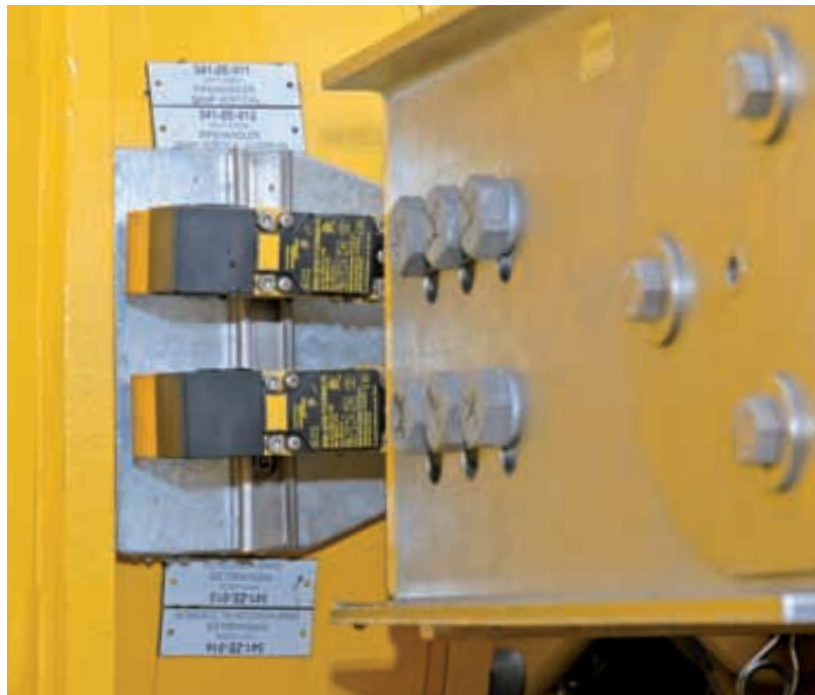
To be able to operate two inductive sensors in close proximity, Turck developed a sensor with a shifted oscillator frequency
