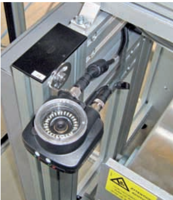
The DataMatrix/Barcode reader from the iVu family reads the code from the back of the figure
