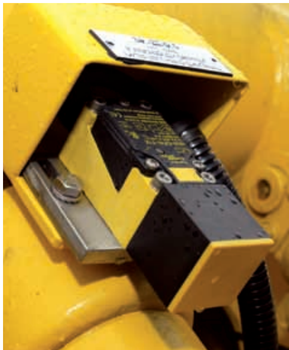
The ATEX-certified Namur-sensors from Turck have to defy the weather conditions of the ocean
