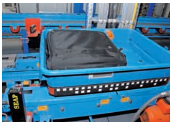
Foolproof identification: The code-reading station from Turck reads the reflector's code at the left side of the chassis
