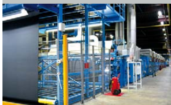
Vebe Floorcoverings uses EZ-Array light curtains to measure with ten times greater accuracy the width of carpet runs at a rate of 35 m/min. Page 26
