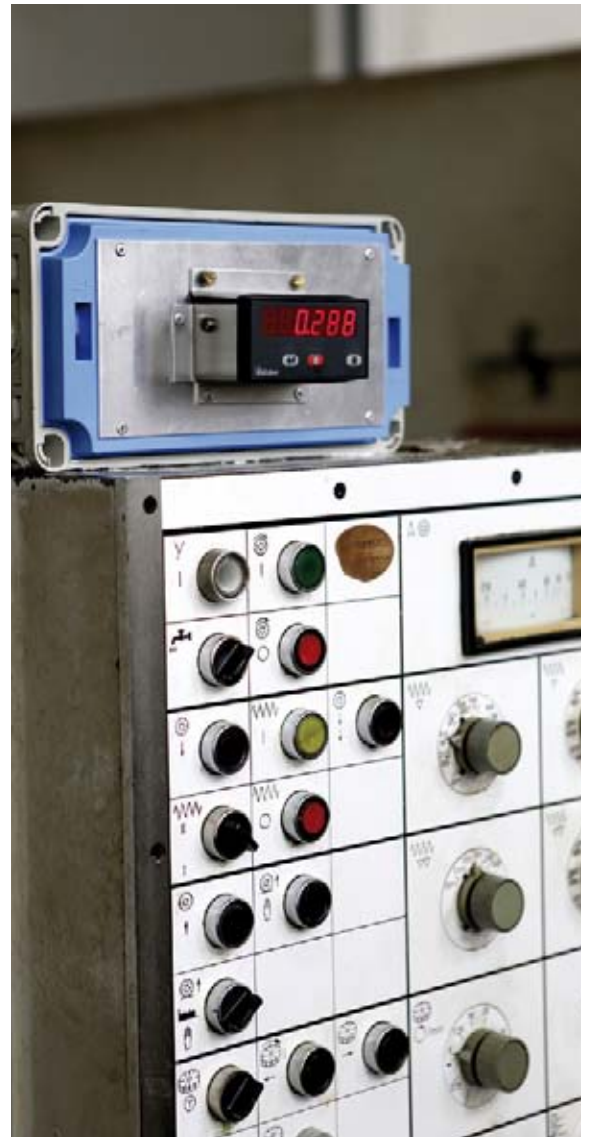
The digital display on the control console of the machine shows the measured value of the LI sensor
