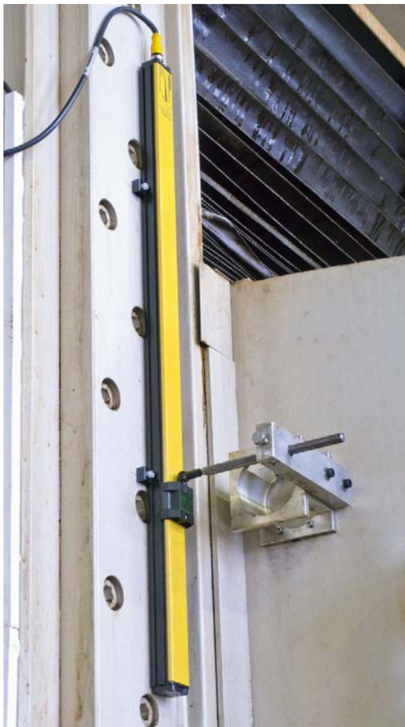
EMC immune: The 30 kW electric motor of the main spindle fitted behind the bellows does not disturb Turck's LI-Q25 in the slightest
