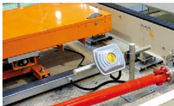
Turck's BL ident UHF-RFID system detects the data carriers on the individual car body parts at a Chinese car manufacturer. Page 18
