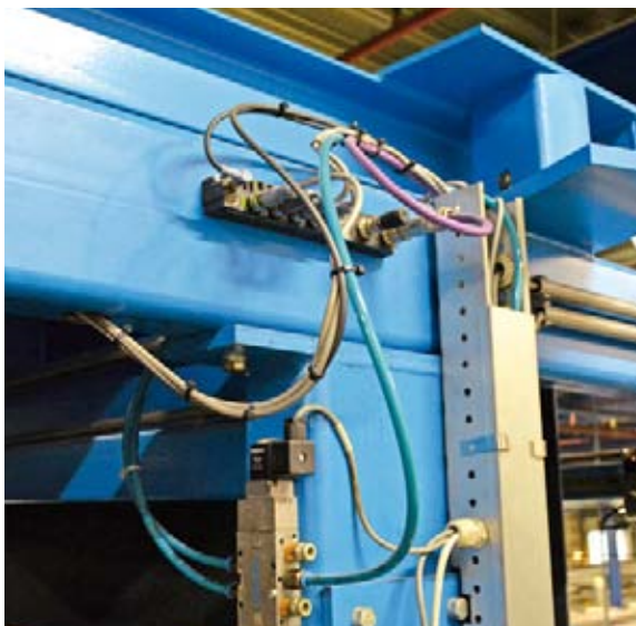
Turck's block I/O module brings the digital measuring signals to the controller via IO-Link and Profibus
