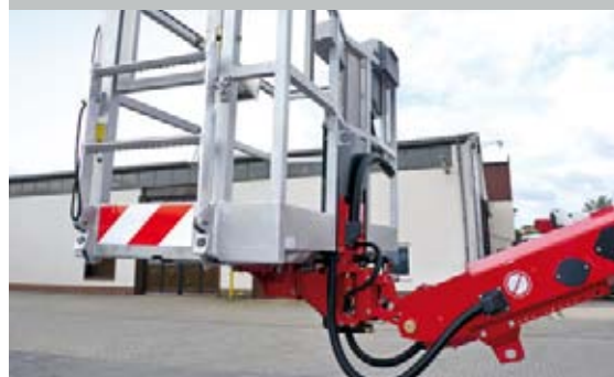
Ruthmann has fitted STEIGER® aerial platforms with Turck's Ri360 inductive angle sensor for measuring the swivel angle of the working cage. Page 28
