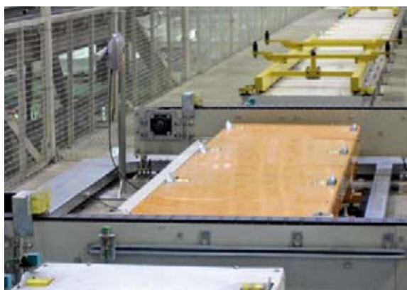
The body parts on the rail are later reliably captured by UHF-read/write head
