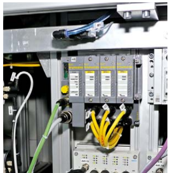
The data of the read/write heads reaches the database using Turck’s BL67 gateway with RFID modules
