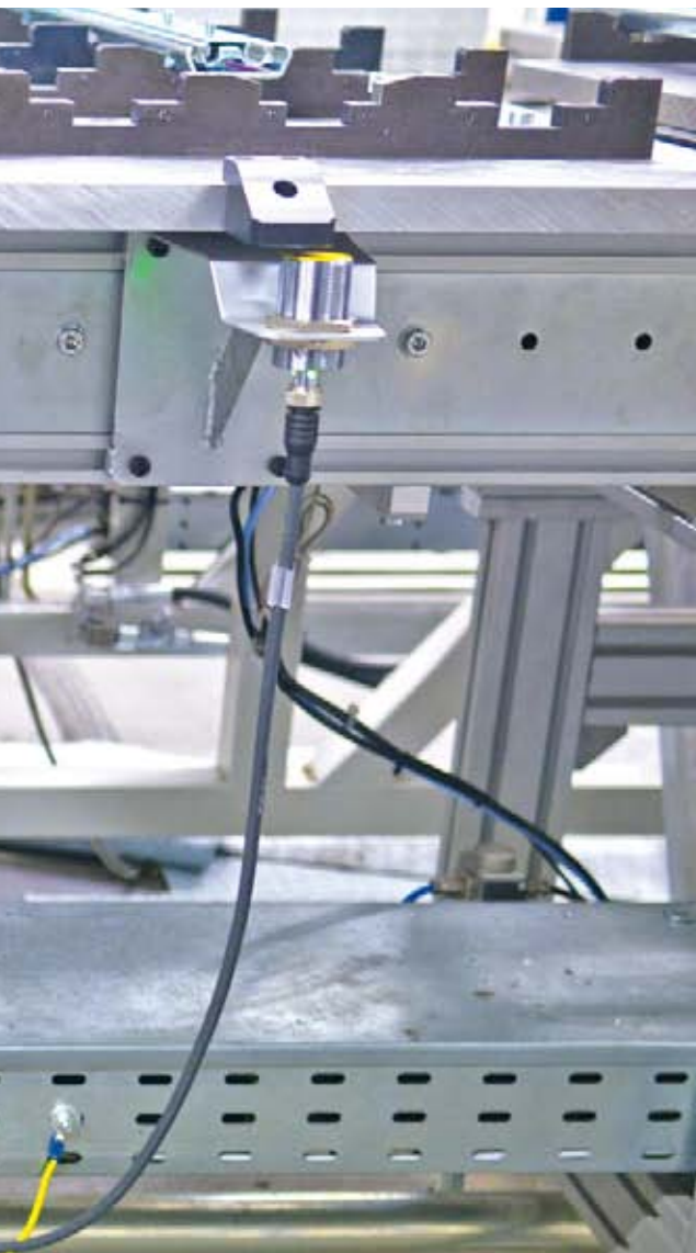
The tag was fitted to the workpiece carrier with the black plastic holder
