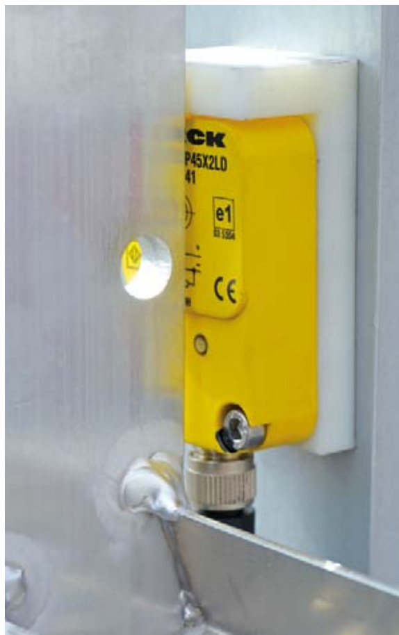
The Bi20-Q20 detects the folded ladder on the outer wall of the working cage
