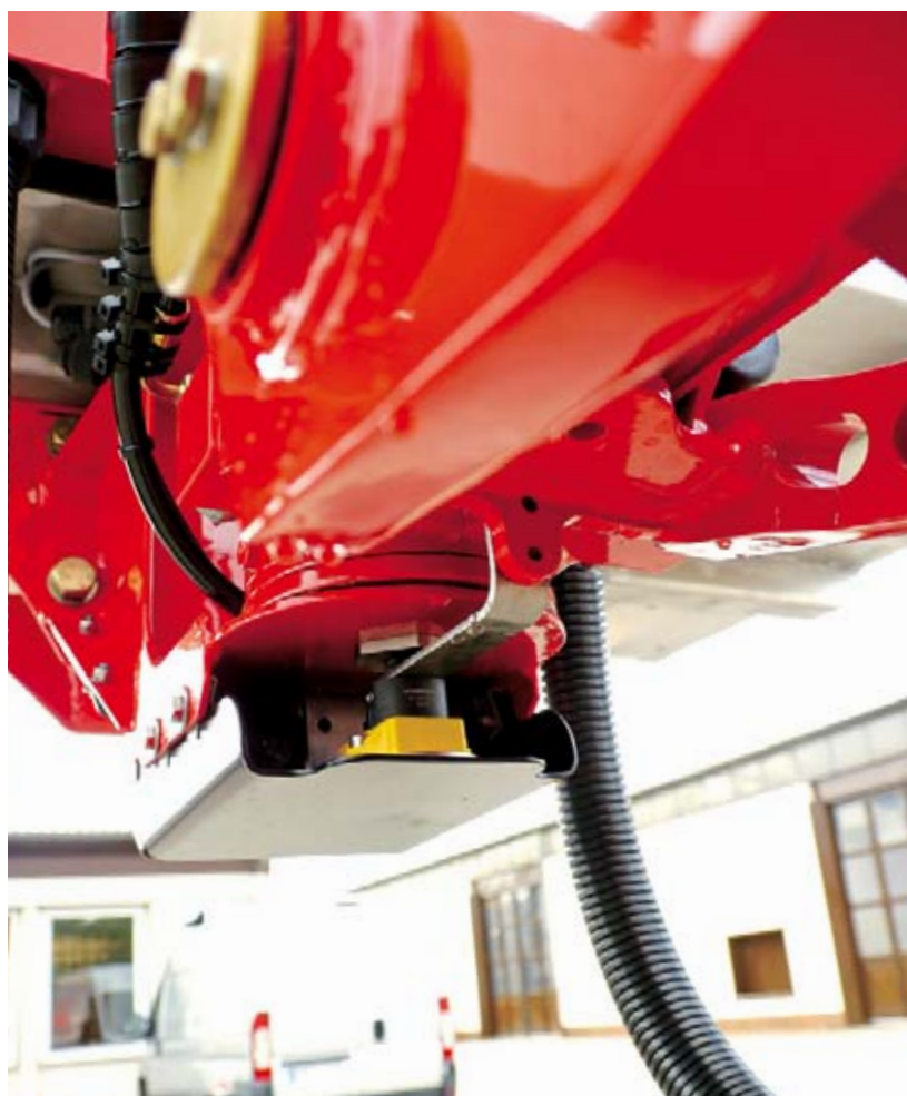
The compact Ri360-QR14 is reliably protected from mechanical damage by the steel cover
