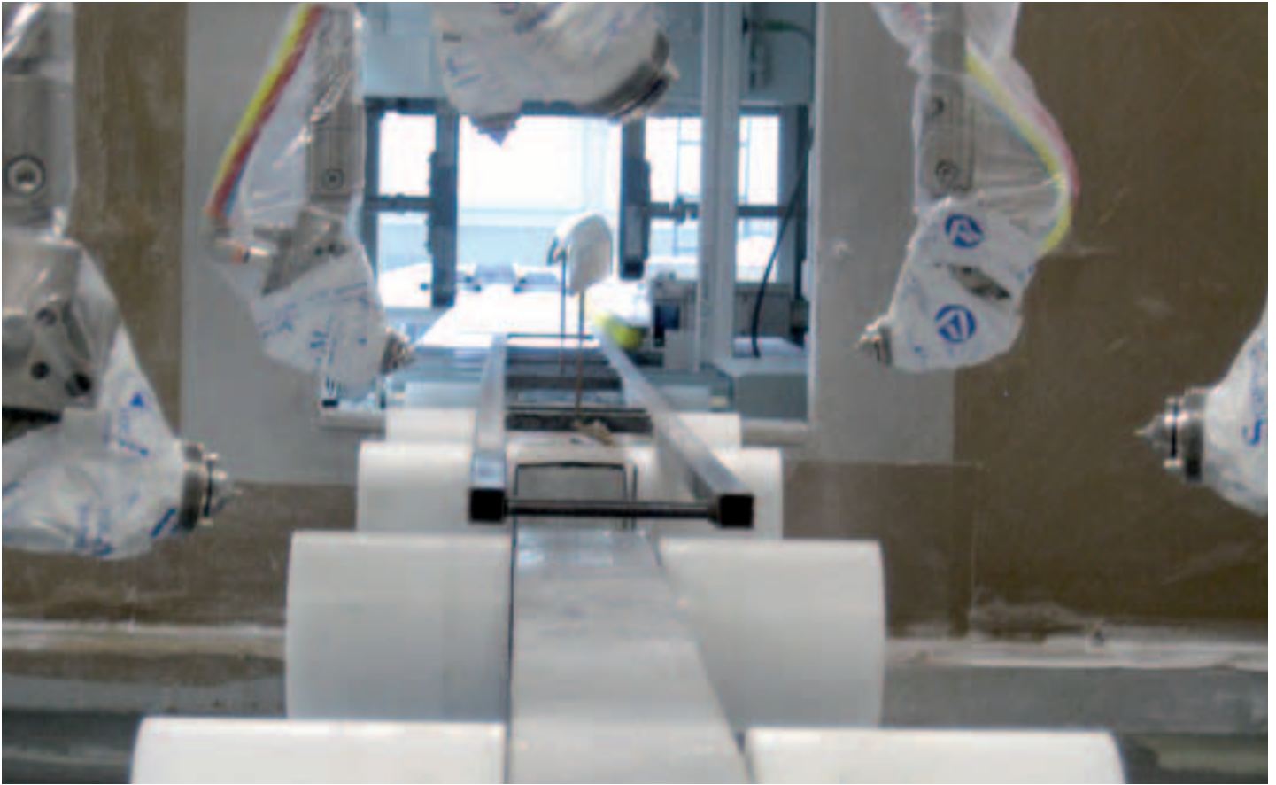
The molding on the parts carrier is directly blocked by the controller so that the contour of the molding is correctly recorded
