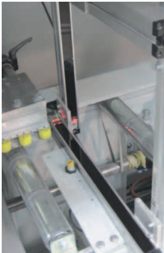
The EZ Arrays have an integrated controller
