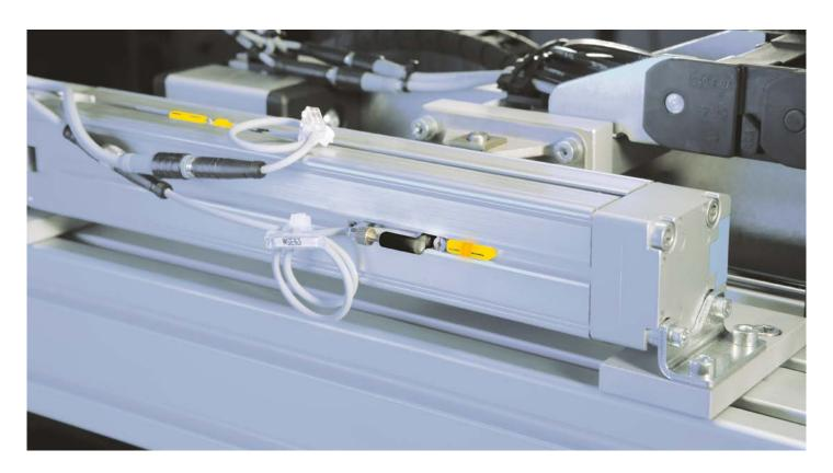
You can now query the piston position on standard pneumatic cylinders very comfortable with a single sensor type. The new magnetic field sensors BIM-UNT, BIM-UNTK, BIM-UNR and BIM-UNC by Turck not only support efficient standardization, they also offer more leeway for optimization in terms of construction, purchase, production, operation and service. Use the unique performance spectrum of these sensors and reduce your application costs effectively.
