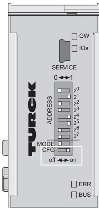
Fig. 18: DIP-switch for storing the station configuration
