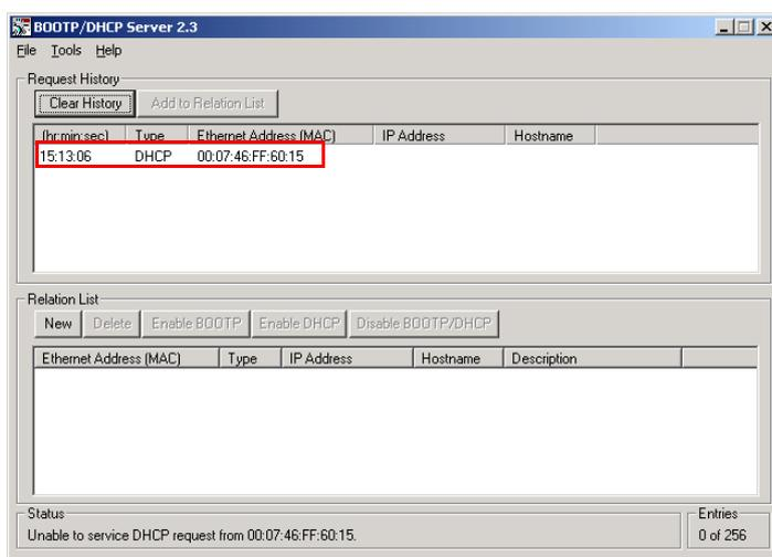
Fig. 120: DHCP-request of the device
