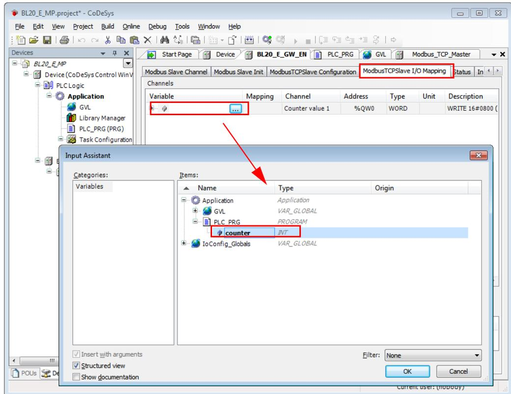
Fig. 68: Mapping of the counter value to %QW0
