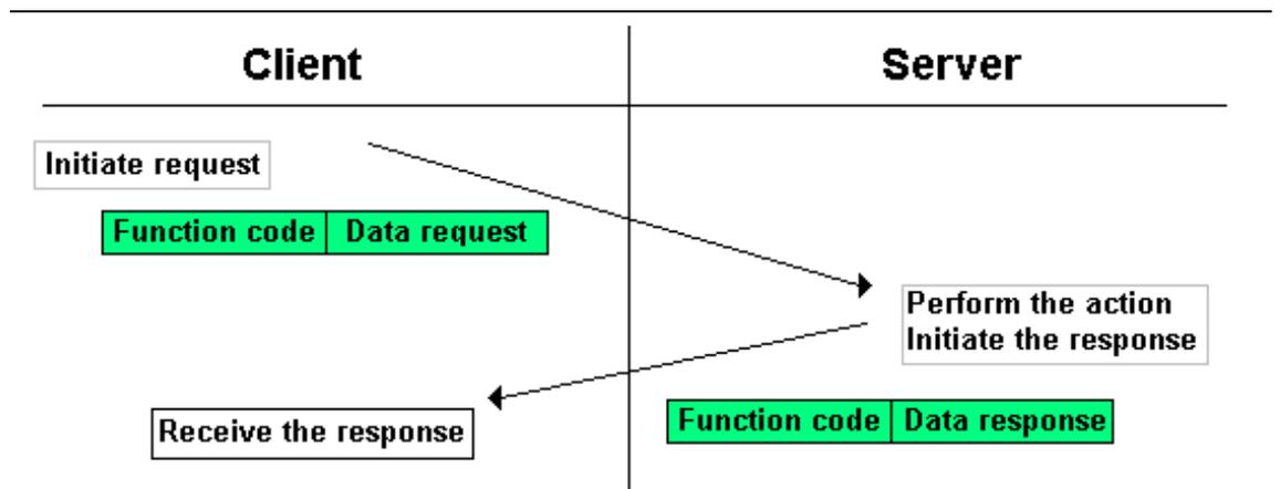
Fig. 47: Modbus data transmission (acc. to Modbus-IDA)
