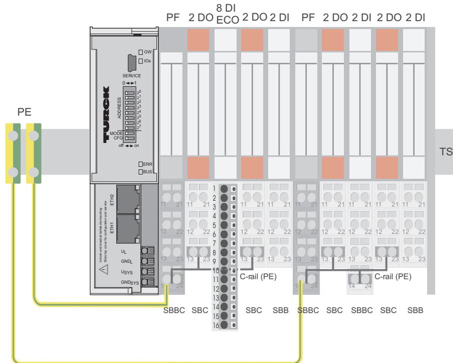
Fig. 112: Using the C-rail as a protective earth
