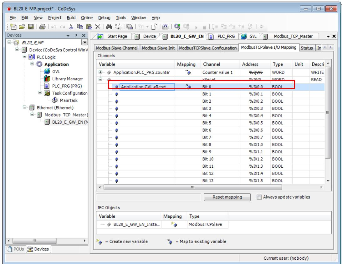
Fig. 71: Mapping of "xReset" to bit %IX0.0
