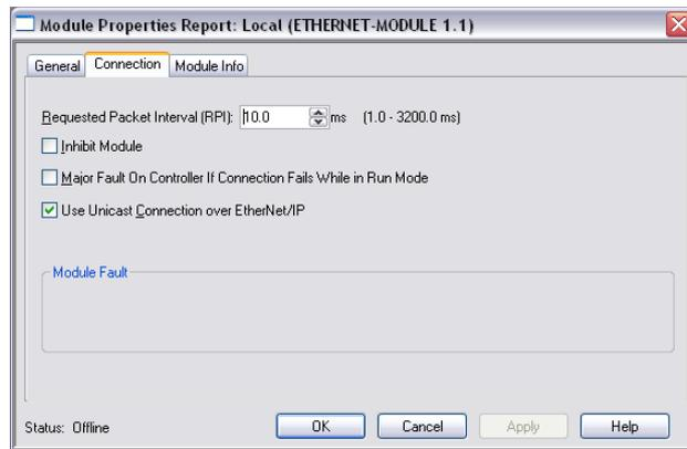
Fig. 34: Set connection options for the gateway
