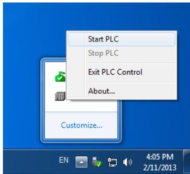
Fig. 77: Starting the WIN V3-PLC
