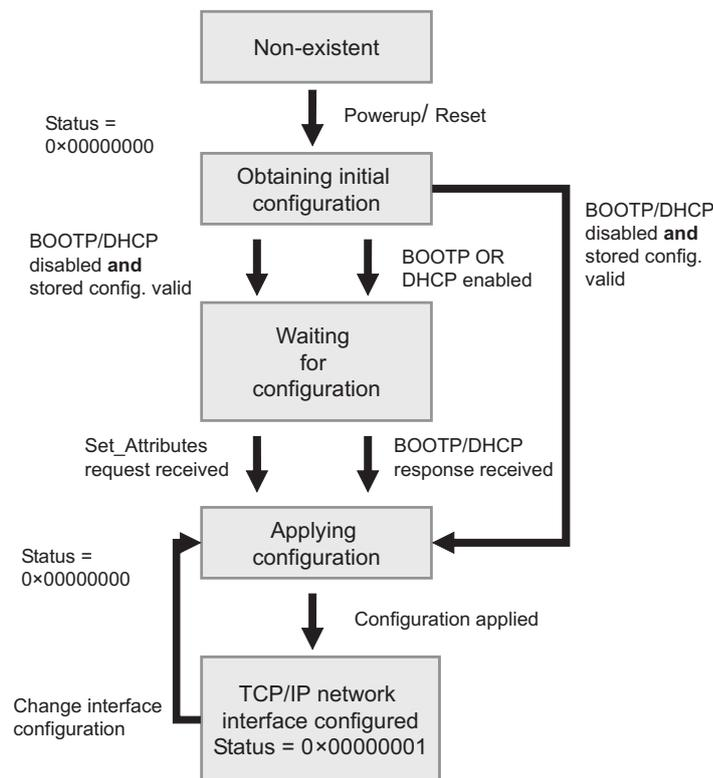
Fig. 29: TCP/IP object state diagram (acc. to CIP Spec., Vol.2, Rev. 1.1)
