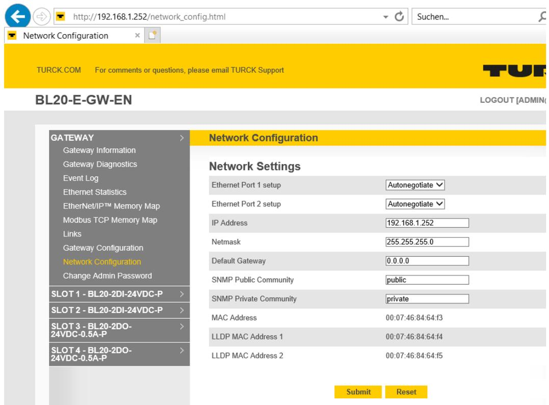
Fig. 16: Web server with Network Configuration
