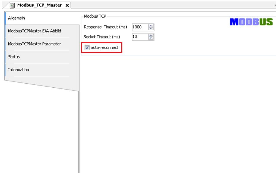
Fig. 59: Parameterization of the Modbus TCP-Master
