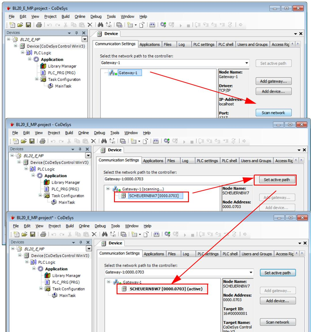
Fig. 56: Setting the communication path
