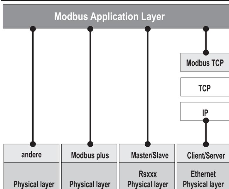
Fig. 45: Schematic representation of the Modbus Communication Stack
