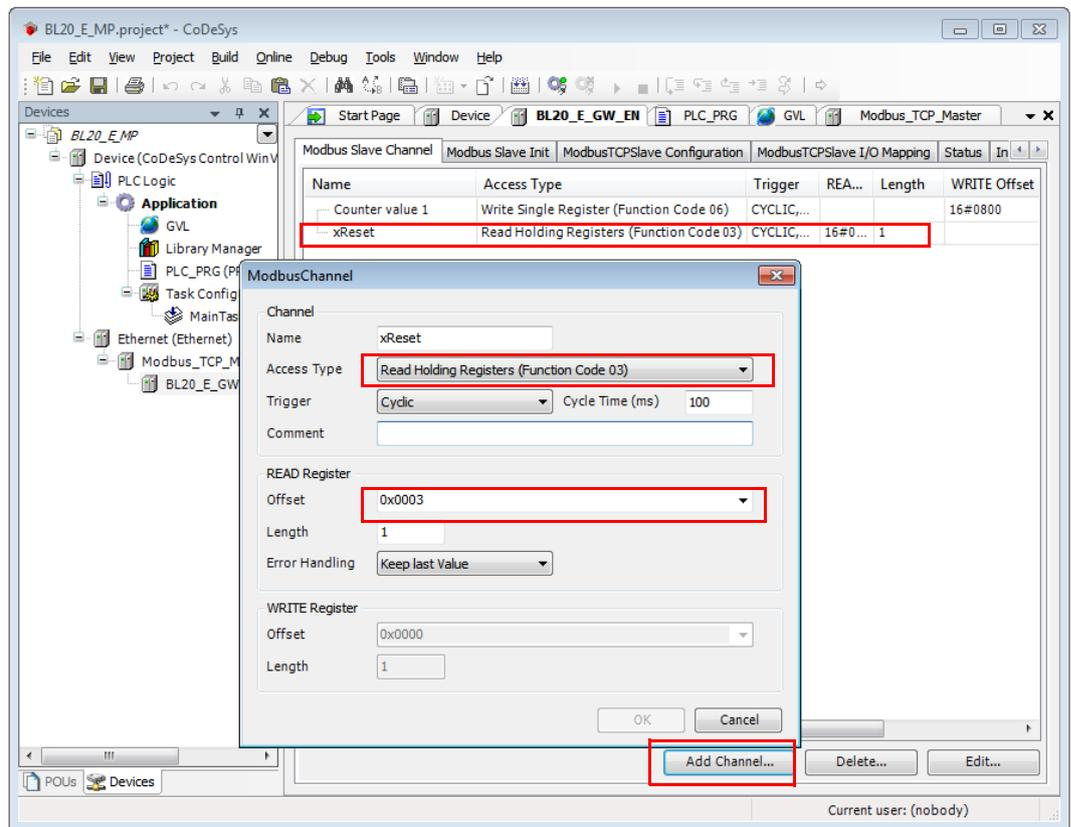
Fig. 70: Modbus channel, read "xReset", FC03
