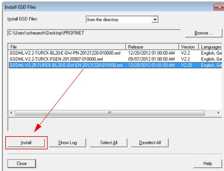
Fig. 92: Install GSD files
