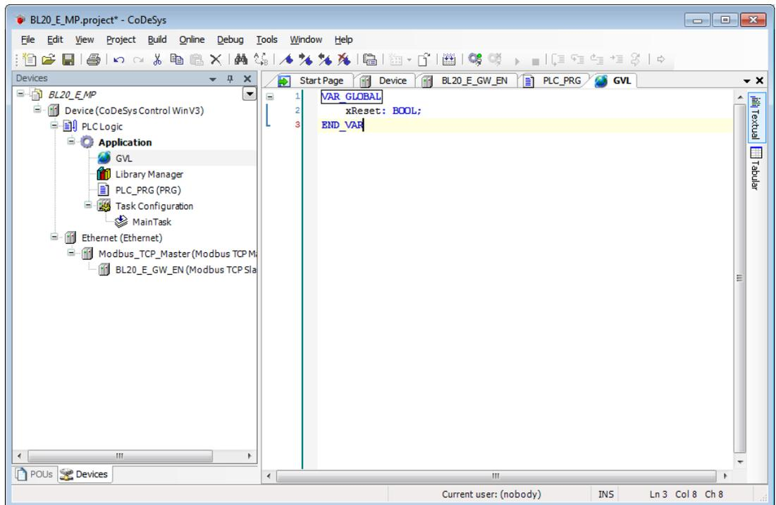
Fig. 62: Example for the definition of a global variable
