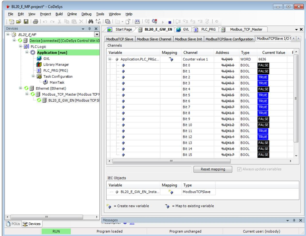
Fig. 81: Modbus TCP Slave I/O image with process data
