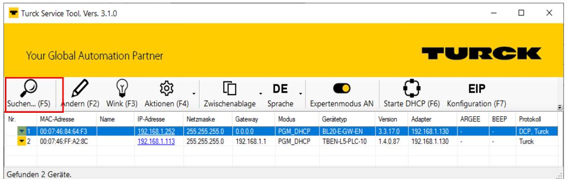
Abb. 23: IP-Address Tool, search function
