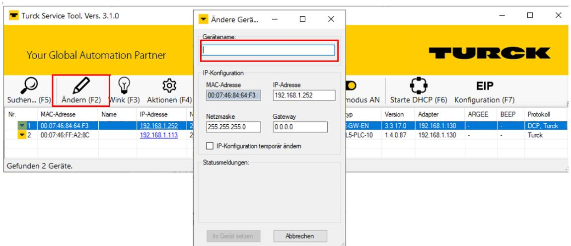
Abb. 26: IP Address Tool, PROFINET name assignment
