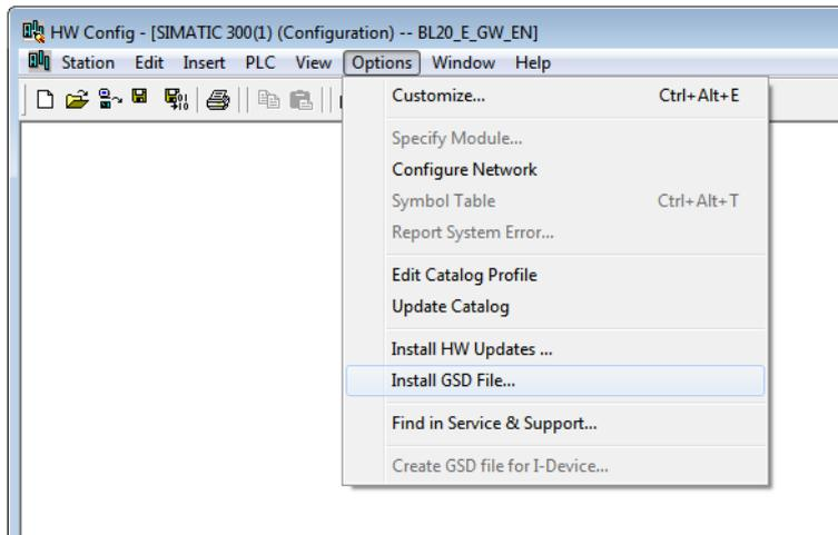
Fig. 91: GSD files install
