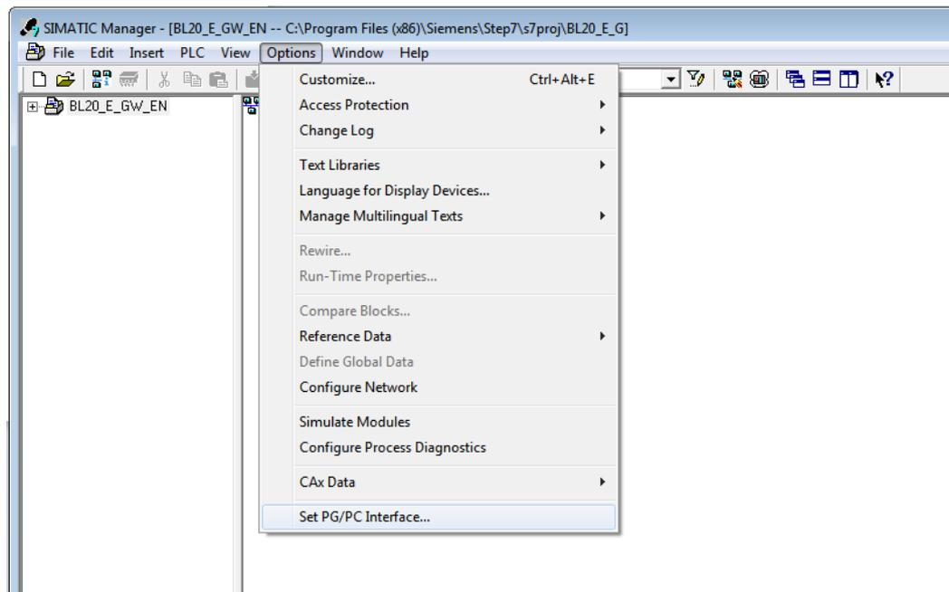
Fig. 90: Command "Set PG/PC Interface..."
