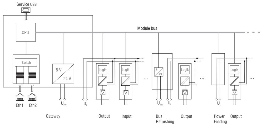
Fig. 114: Block diagram of a BL20 station with BL20-E-GW-EN
