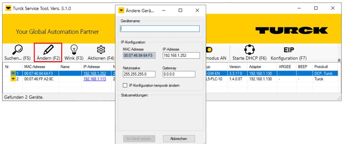
Abb. 24: IP-Address Tool, Changing IP Properties
