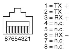
Fig. 5: RJ45 female connector
