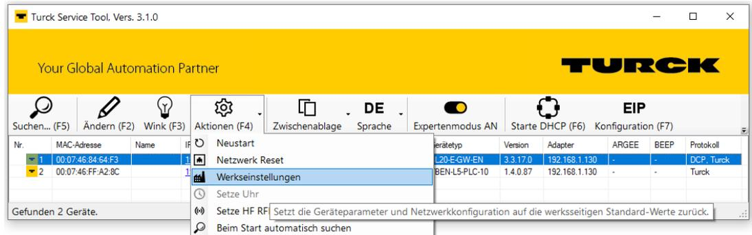
Abb. 27: IP Address Tool, reset to factory settings
