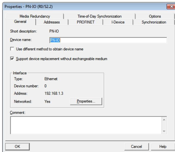
Fig. 103: Settings of the PROFINET-controller
