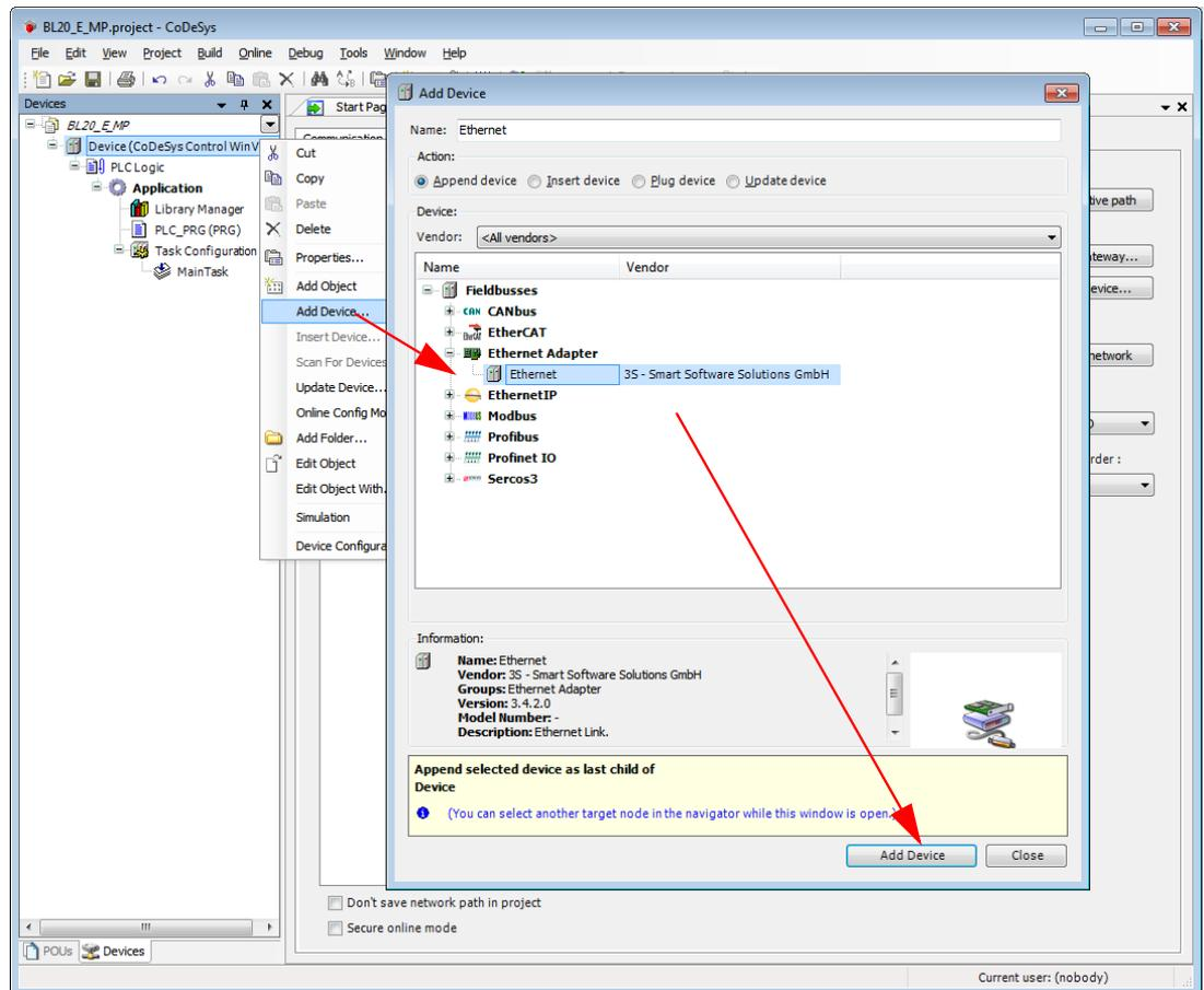
Fig. 57: Adding the Ethernet Adapter as device
