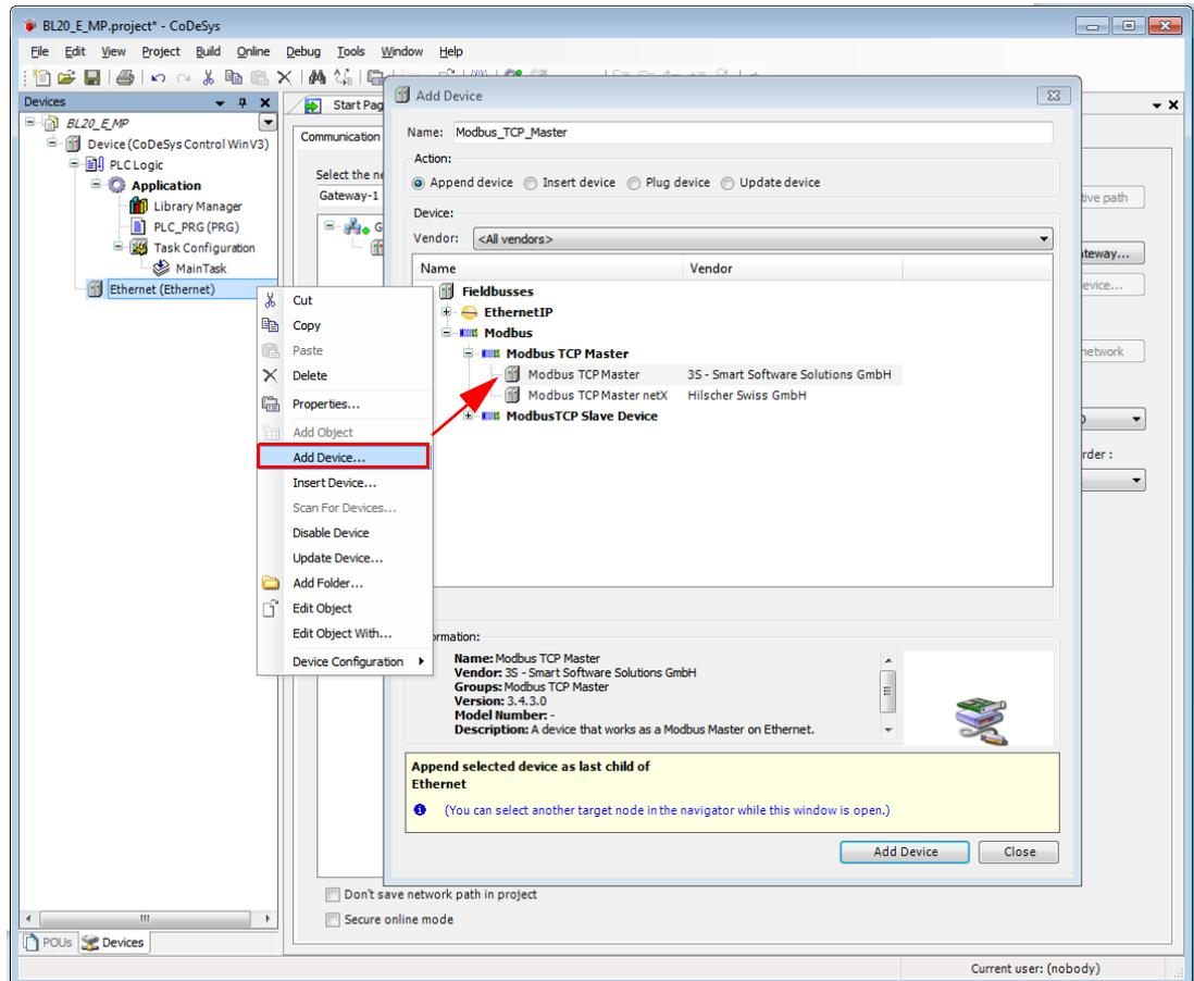
Fig. 58: Adding the Modbus master
