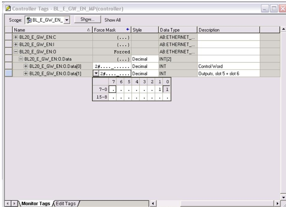
Fig. 42: Setting outputs at BL20-2DO-24VDC-0.5A-P
