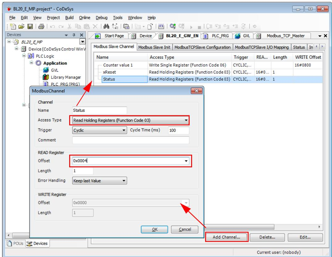
Fig. 73: Setting the Modbus channel for reading the status word
