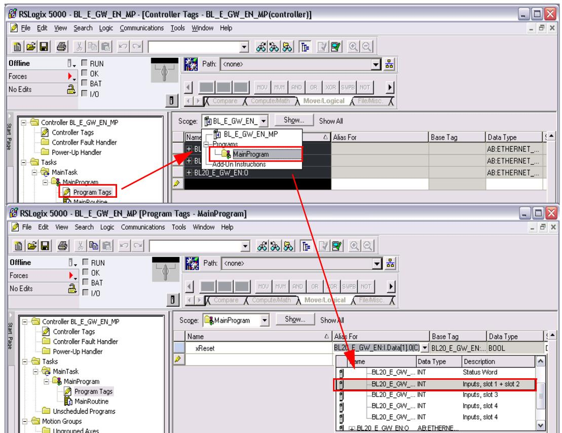
Fig. 44: Definition and mapping of xReset
