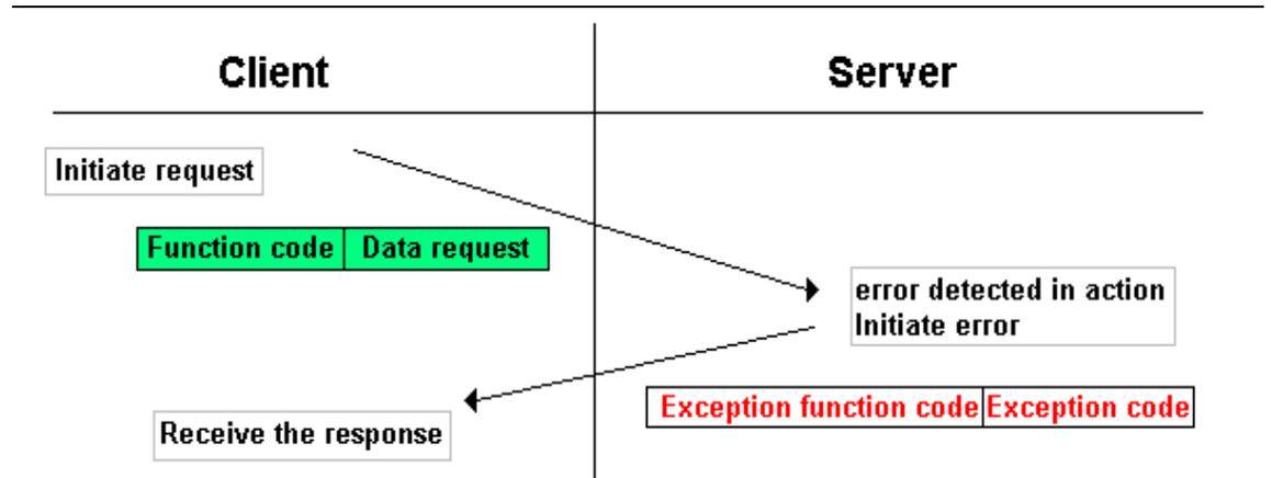
Fig. 48: Modbus data transmission (acc. to Modbus-IDA)
