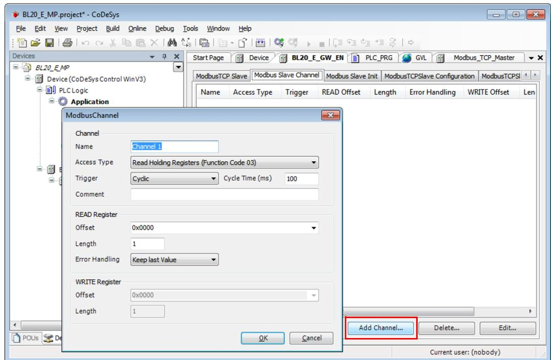
Fig. 63: Setting the Modbus channels, examples
