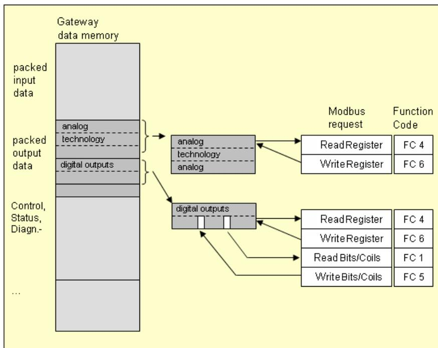
Fig. 49: Picture of the data memory of the BL20 modules
