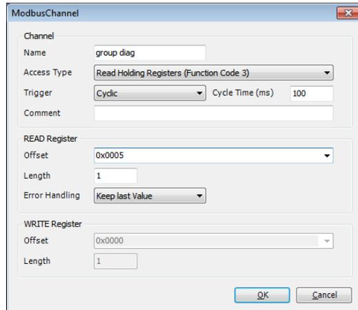
Fig. 84: Channel for reading out the group diagnosis
