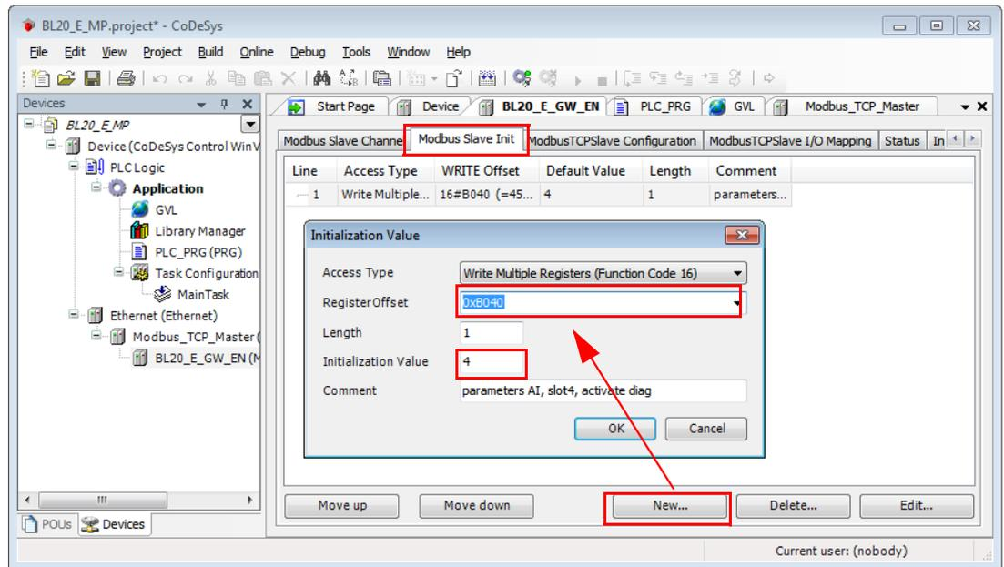
Fig. 76: Setting the initialization channel for the parameterization
