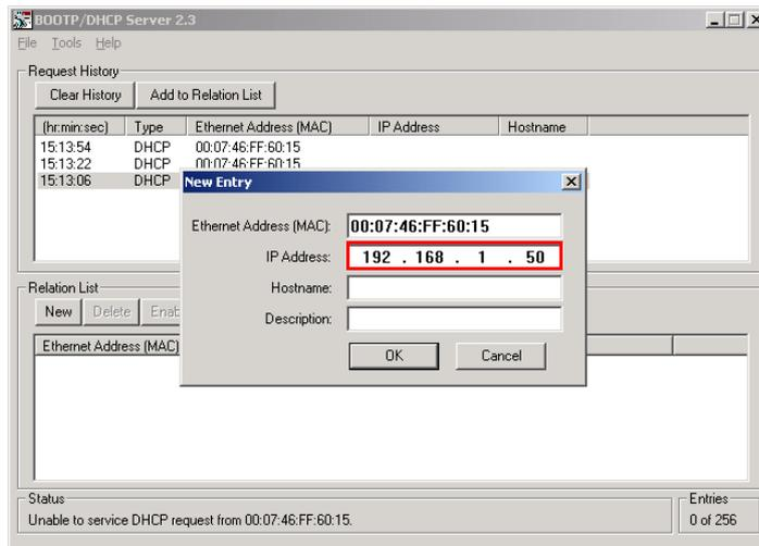
Fig. 121: Setting the IP address via DHCP
