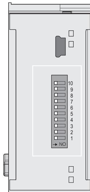
Fig. 6: DIP-switches at the gateway
