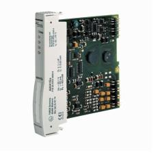
The input module AIH41Ex is used for the connection of 4-wire transducers (passive input = sink mode / transducer active).
