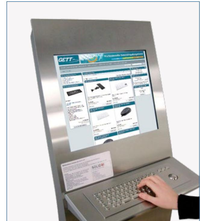
*InduSteel<sup>2</sup> keyboards are used in SOLIDD terminals (pictured above). With a compact layout of 68 clearly arranged keys, the stainless steel keyboard is optimized for the operation of web-focused applications.*
