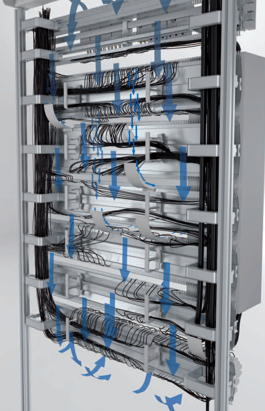
Schematic view of the air flow at the back of the LSC AirSTREAM frame
