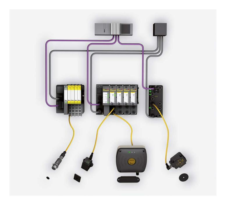
BL ident® is an all-in-one modular RFID system that plays out its strengths in the food industry. The TURCK I/O systems BL67 (field), BL20 (cabinet) and BL compact (field) are the basic components of the modular concept. Both technologies, HF (13.56 MHz, ISO15693) and UHF (865...928 MHz, acc. to ISO 18000-6C/EPCglobal Class 1 Gen 2) are available in one identification solution.
