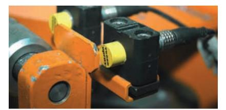
One for all: Turck's ferrite-coreless uprox+ sensors have the same high switching distance on all metals
