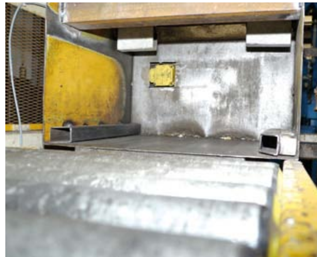
The read/write head at the feeding recognizes if the right batch is supplied to the blasting machine
