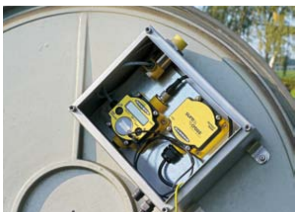
The IP67 components of the DX80 system including sensors are installed in a switchbox
