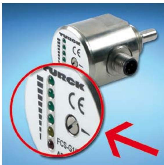
The FCS immersion sensor can be adjusted onsite with the help of the LED display and the potentiometer
