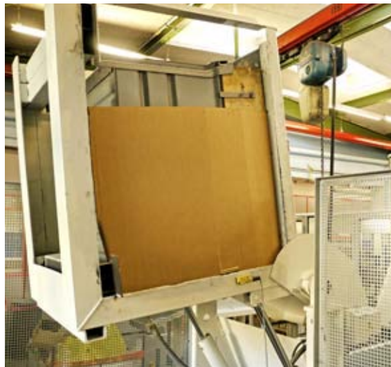
The inclination sensor at the feeding gives a signal when the box is emptied
