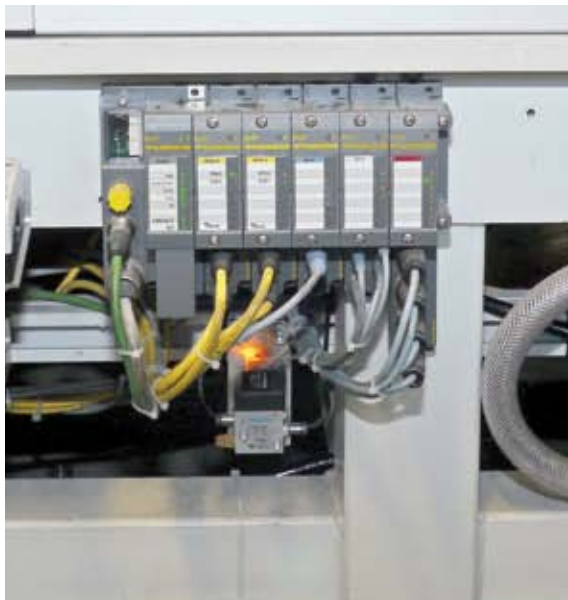
The read/write head at the feeding recognizes if the right batch is supplied to the blasting machine
